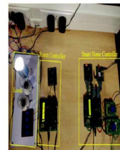
Figure 2: Domestic Energy Management System with proposed smart Home Controller.
