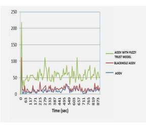
In figure. 3. The black hole attacked AODV is increased compare to normal AODV and AODV fuzzy trust model packet delivery ratio is high compare to both the normal AODV and black hole attacked AODV. This shows the fuzzy trust model make more packet delivery ratio. Though the packet delivery ratio is higher in proposed routing, end to end delay is less and throughput is significantly improved by the proposed trust routing.
