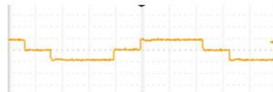
Fig 15 Output waveforms showing 2 steps at 4 Vp-p input signal
