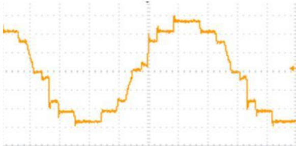
Fig17. Output waveforms showing 4 steps at 6 Vp-p input signal
