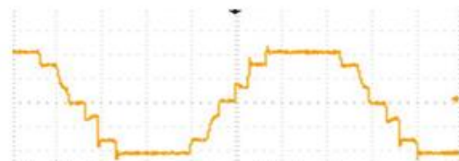
Fig 16. Output waveforms showing 3 steps at 5 Vp-p input signal.
