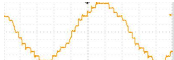
Fig 19. Output waveform showing 6 steps at 8 Vp-p input signal
