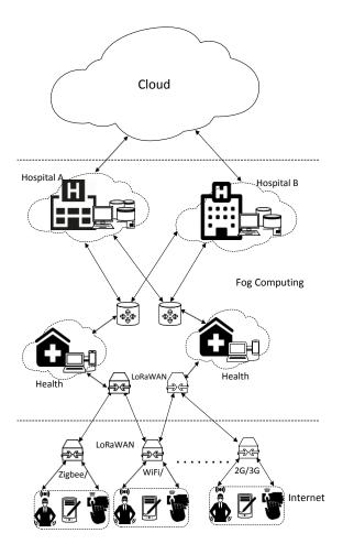
Figure 2: IOT and Fog based health monitoring system.
