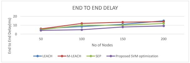
Figure 7 End to End Delay comparison between the proposed routing protocols @Area Dimension 80x160Sq.meters
