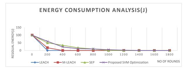
Figure 4 Energy Consumption Analysis for the various protocols at Area of Dimension 100x200 Sq.meters(20000Sq.meters)
