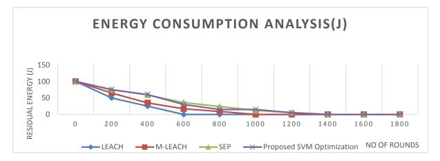
Figure 2 Energy Consumption Analysis for the various protocols at Area of Dimension 60x120 Sq. meters (7200Sq.meters)
